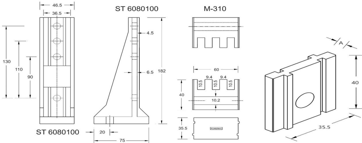
Our Busbar Supports are moulded from a flame retardant and track resistance glass reinforced Thermoset Polyester compound recognized to use for current carrying devices under UL Material Recognition No. E249670.
