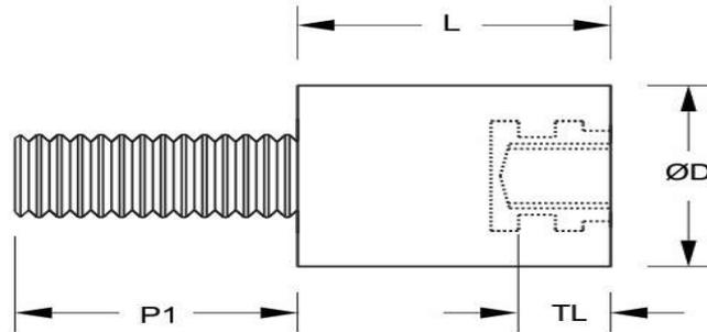
**Our Insulators are moulded from a flame retardant and track resistance glass reinforced Thermoset Polyester compound recognized to use for current carrying devices under UL Material Recognition No. E249670 & products are itself certified under UL Product Recognition no. E314972.**
